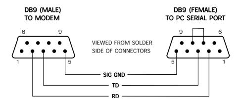
Make up this lead to connect the RTM2400 modem to a PC serial port. Use a program such as Terminal for Windows® to send AT Commands to the modem. (see *AT Commands. Page 14*).
